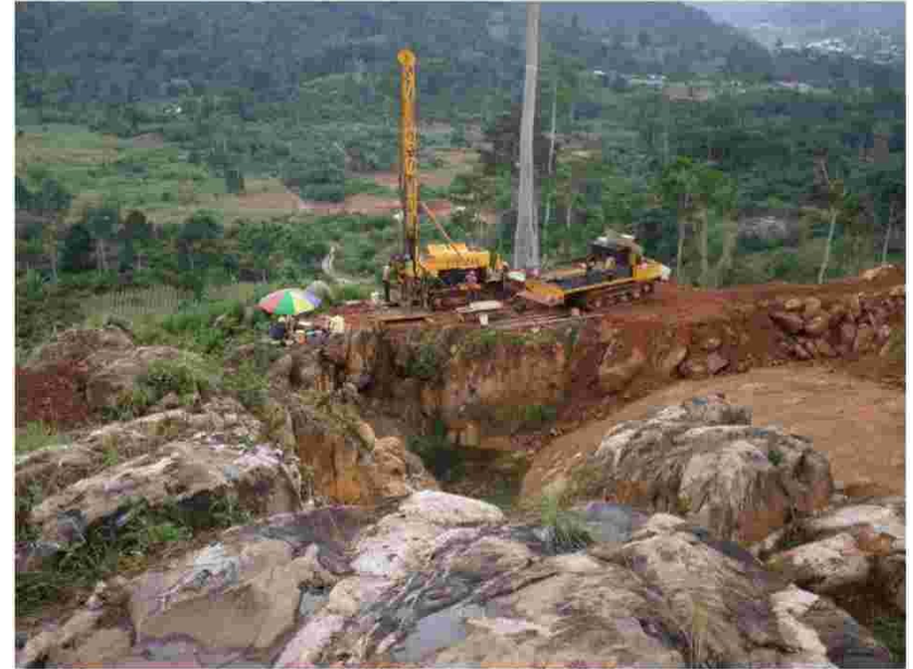
Diamond Core Drilling on High Grade Shoot – Borehole #CCDD16013 (Facing SW)
